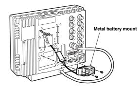
**3** Fix the V-mount type battery holder with four screws (length 8 mm) supplied with the holder, and then fasten the two screws on the terminal section.
